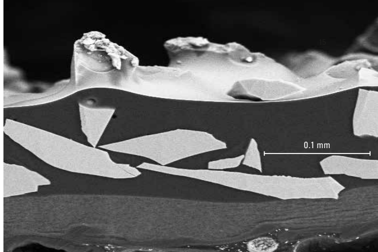
Cross section of SiC abrasive paper
