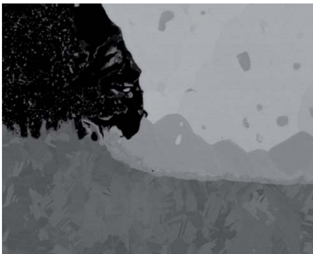
Solder ball after ion beam polishing
