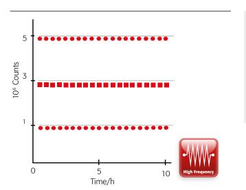
Superb long-term signal stability for all emission lines offered by the High-Frequency Generator: Li 670 nm (♠), Mn 257 nm (■), Al 396 nm (♠)
