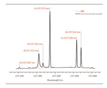
Automatically fitting a baseline to any spectrum the ABC is a revelation in data evaluation.
