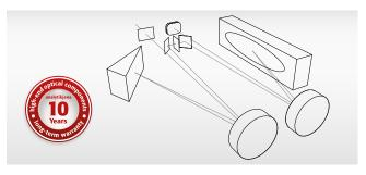
A compact ensemble of high-end optical components yields the unrivalled resolving power of the PlasmaQuant® PQ 9000 Elite.
