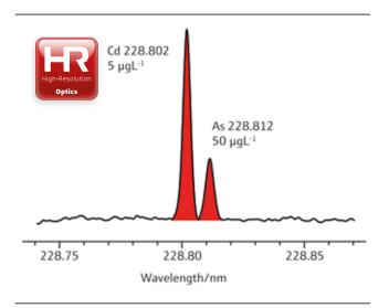
Only a few picometers apart the Cadmium and Arsenic line are well-separated and can be used analytically without difficulty.
