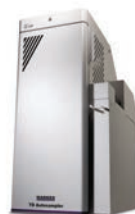
Markes TD100 Cryogen-free re-focusing with 100 sample capacity
