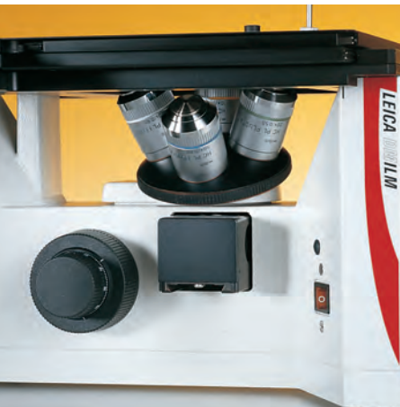
Central part of the microscope with quadruple objective nosepiece, reflector slide, focus control
