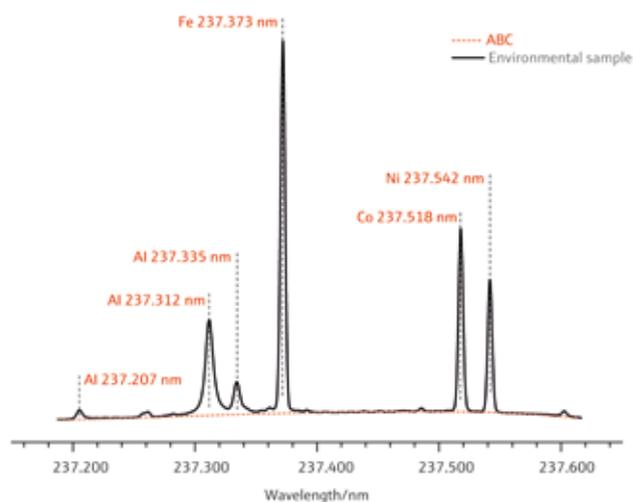
Automatically fitting a baseline to any spectrum the ABC is a revelation in data evaluation.
