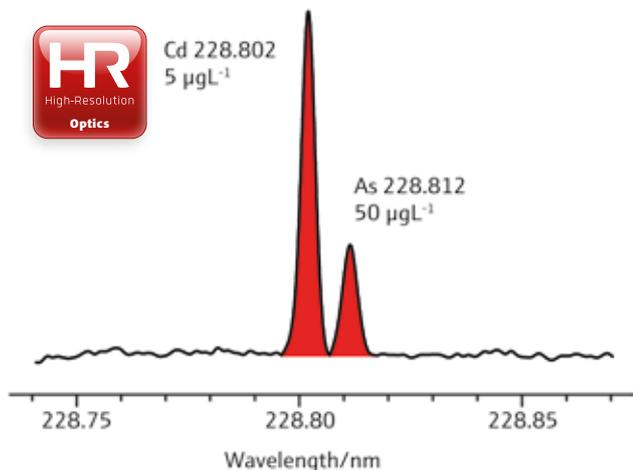
Only a few picometers apart the Cadmium and Arsenic line are well-separated and can be used analytically without difficulty.
